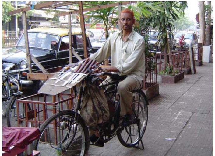
Some ad-hoc jobs are admittedly enterprising, e.g., this knife sharpener using the rear wheel of his stationary bike as a sharpening device and mobile office.
